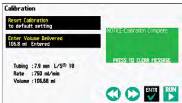
Tubing calibration procedure for precise accuracy
