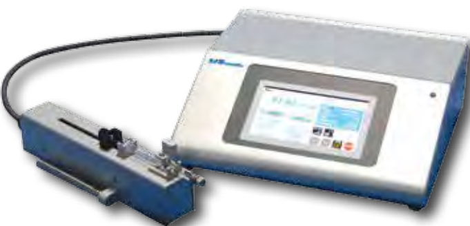
Legato ® 130 Single Syringe Nanoliter Infuse/Withdraw Pump
